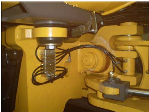
Progressive dividers help to ensure lubricant is delivered to high-demand bearings, pins and bushings
