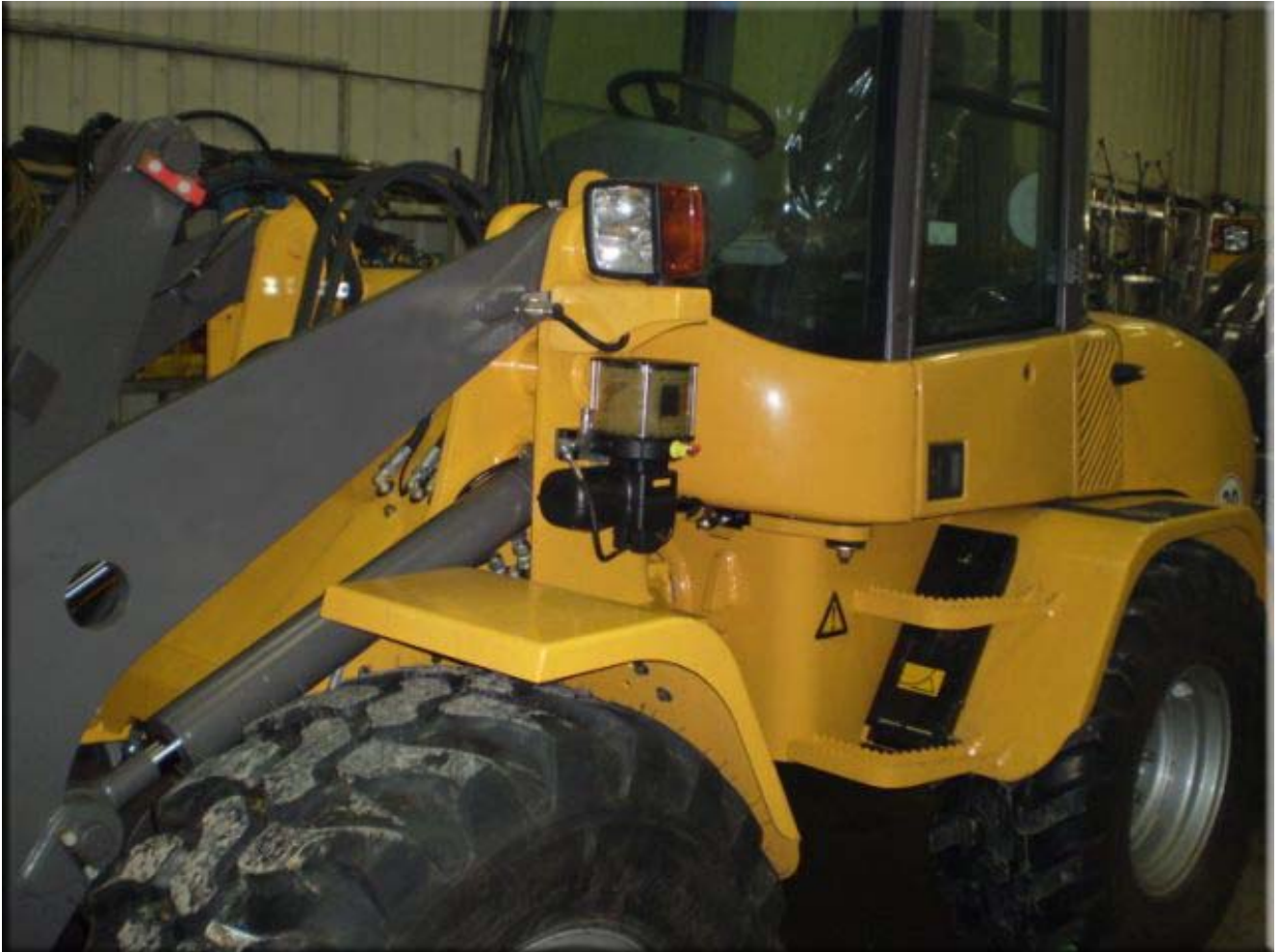
On this wheelloader , an ILC-MAX pump is mounted on the operator deck or near the cab for easily monitoring
