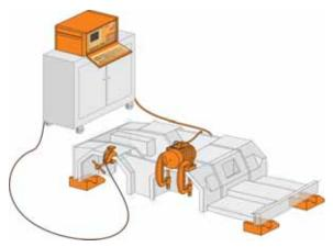
VIBMATIC 6000<sup>®</sup> Vibration stress reduction
