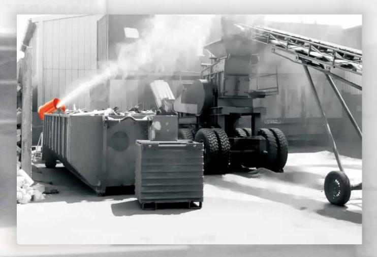
With a working pressure of 16 bar, the DUSTEX<sup>®</sup> Fog Blower creates a fine water fog with the applied nozzles that binds the dust particles directly at the source and reduces visibly the dust emissions.
